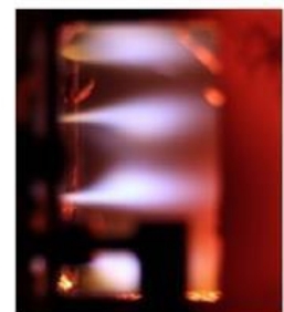
Micro-mix hydrogen flame [FH Aachen]
